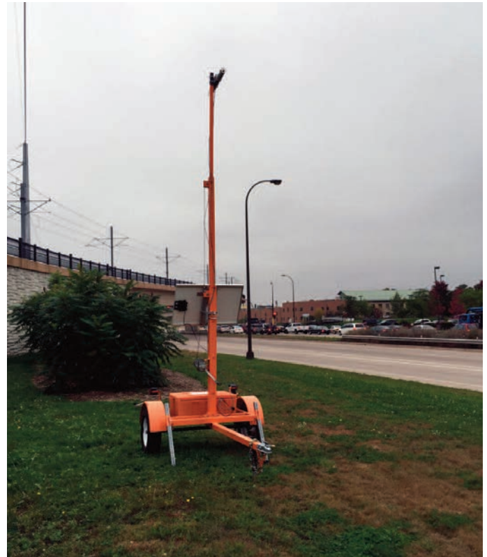
Fig. 1: DATACAR System portable installation including Traffic Radar Sensor and 3000CP unit
