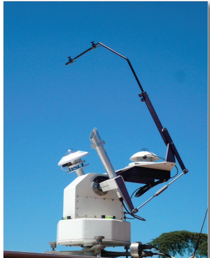
Meteorological Station with SunTracker-3000
