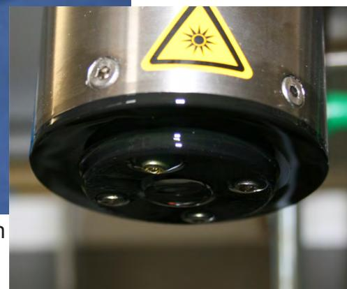
A new innovative nano-coating on the optical lens prevents oil-films and fouling
