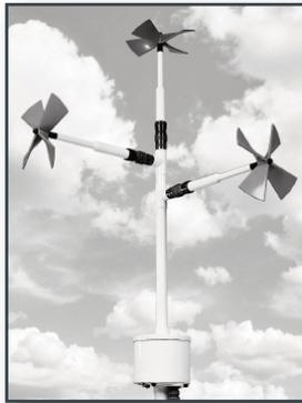
The three Propeller Anemometer sensors are mounted at right angles on a common mast. Each sensor measures the wind component parallel with its axis of rotation. Propeller response as a function of wind angle approximates the cosine law, allowing true wind velocity and direction to be calculated.
