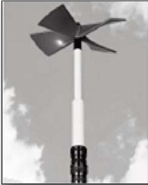
The Propeller Anemometer is especially suited for measuring the vertical wind component. Since normal wind direction seldom exceeds  $\pm 30^\circ$  from horizontal, propeller response can be calibrated to follow the cosine law within 3% over this range.
