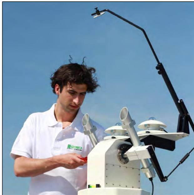
***Model SunTracker-3000 with shadow arm and disc, two Pyrheliometers and two Pyranometers***
