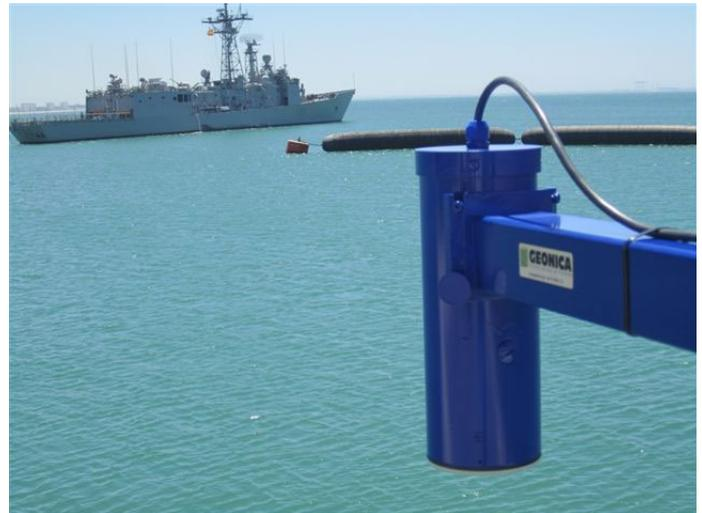
Water Level Sensor Model RADAR-6115
