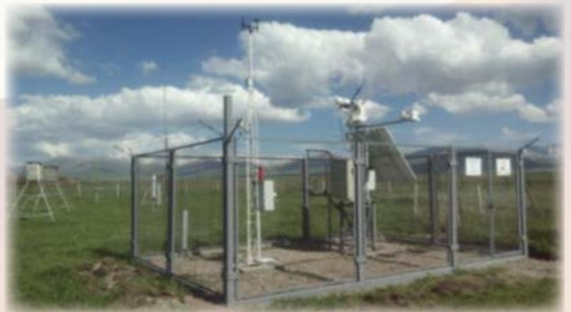
The four stations are based on a **SEMS-3000** with a complete set of meteorological and solar sensors, including the **GEO-SolarSIM-D2**. In addition to Ethernet communications, the station has a 3G/GPRS modem that allows monitoring and downloading of data over the local cellular network.
