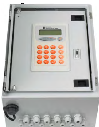
METEODATA Datalogger with Integrated Comms (3G / GPRS, Modbus, Line, Radio or Satellite)
