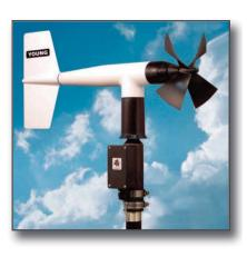
The wind direction sensor is a rugged yet lightweight vane with a sufficiently low aspect ratio to assure good fidelity in fluctuating wind conditions. Vane angle is sensed by a precision potentiometer housed in a sealed chamber. With a known excitation voltage applied to the potentiometer, the output voltage is directly proportional to vane angle. A mounting orientation ring assures correct realignment of the wind direction reference when the instrument is removed for maintenance.
