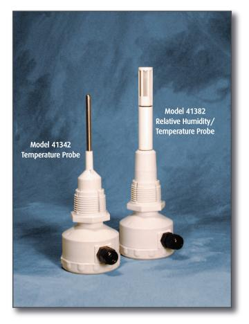
The Model 41382 Relative Humidity/Temperature Probe combines a high accuracy, capacitance type humidity sensor and precision Platinum RTD temperature sensor in one probe. This probe offers a choice of 0-1 VDC or 4-20 mA outputs for T and RH.
