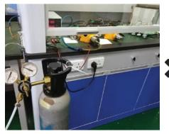
**Factory Calibration** The sensors are bump tested at factory to check their proper functioning for each parameter.
