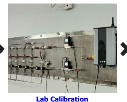
Laboratory calibration is done in a controlled environment for all parameters to compensate for cross-sensitivity and ensure higher data accuracy.
