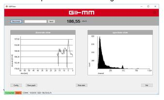
For best reliability the GSP02 uses continuously automatic energy and efficiency calibration by embedded 40K source avoiding false data and alarm.
